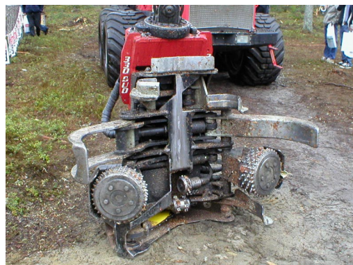
Multi processing head – felling, delimiting, debarking and cross cutting
